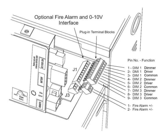
**NOTE** - DALI interface requires the DIM ADJ. to be in the furthest Clockwise (CW) so that the relay opens during Inverter Mode of operation. Dimming requires a DALI signal which the Si125/250W does not provide.
