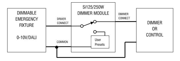
During normal operation, the DIMMABLE EMERGENCY FIXTURE is connected directly to the DIMMER OR CONTROL through the DIMMER MODULE's internal signal relay. Upon loss of power or during a system test, the DIMMER MODULE's internal relay changes state so that the User Presets (5 presets 100% - 20%) will assume control of the dimming level for the DIMMABLE EMERGENCY FIXTURE.
